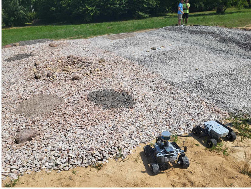
Figure 1: Research field in Józefosław. The field incorporates several key features designed to simulate Martian terrain: a single primary crater formation, four short ripples, one long forked ripple structure, large stones strategically positioned throughout the field, and multiple zones with varying stone granularity.
